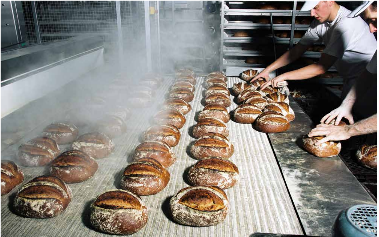
Fresh bread on the balanced wire belt, Type: N 200
