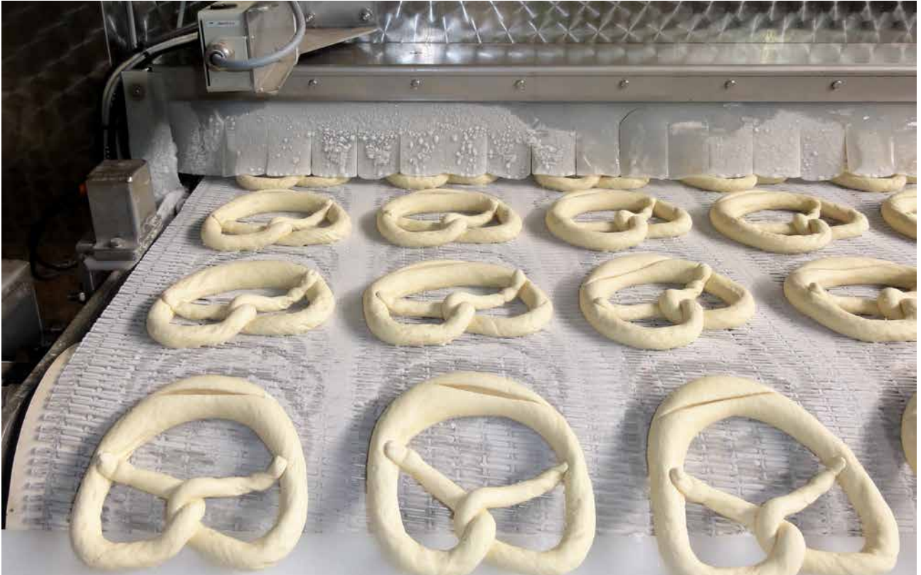
Freezing with cam fabric belt, Type: N 6000
