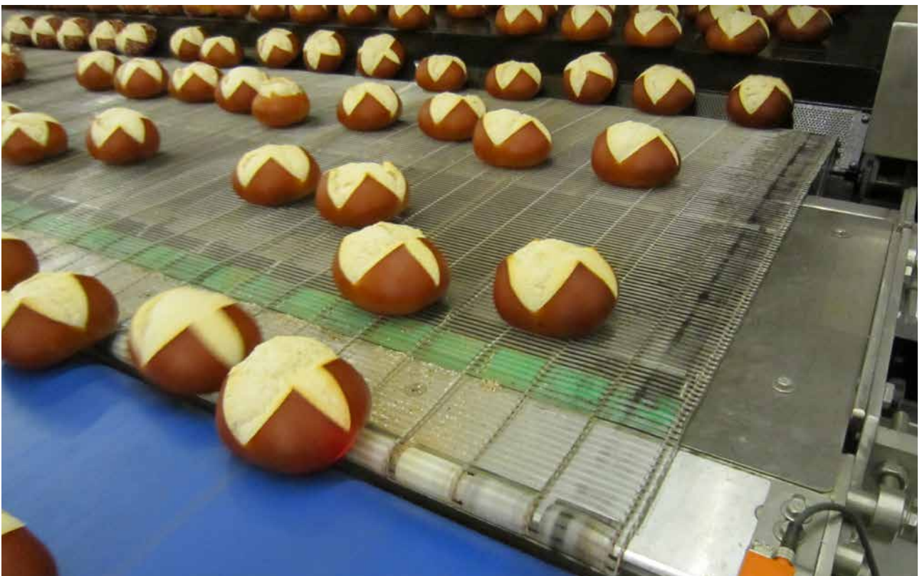
Lye rolls on the rod link belt, Type: N 700
