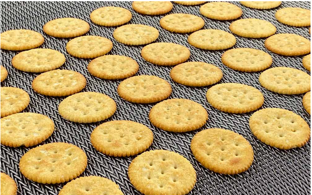
Salt cookies on the balanced wire belt, Type: N 400 V
