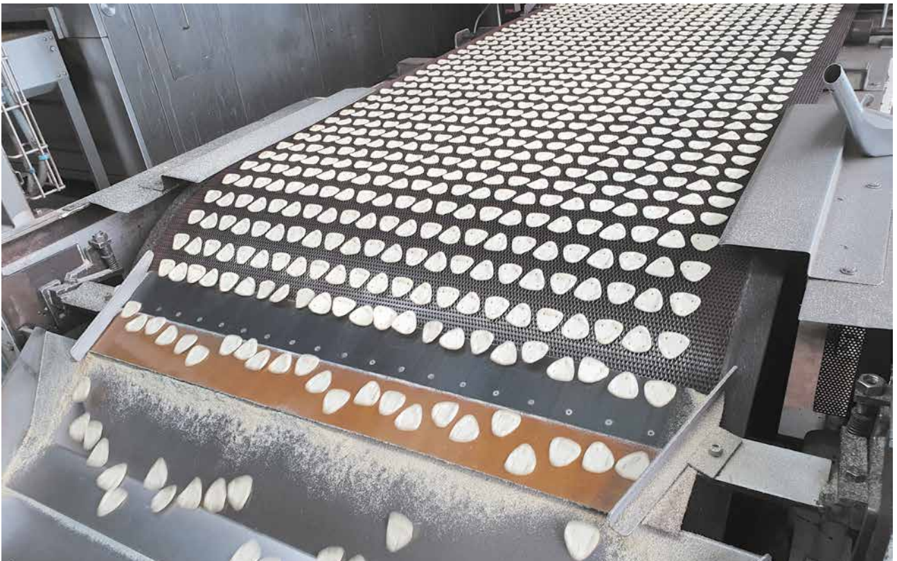
Salt cookies on the balanced wire belt, Type: N 300
