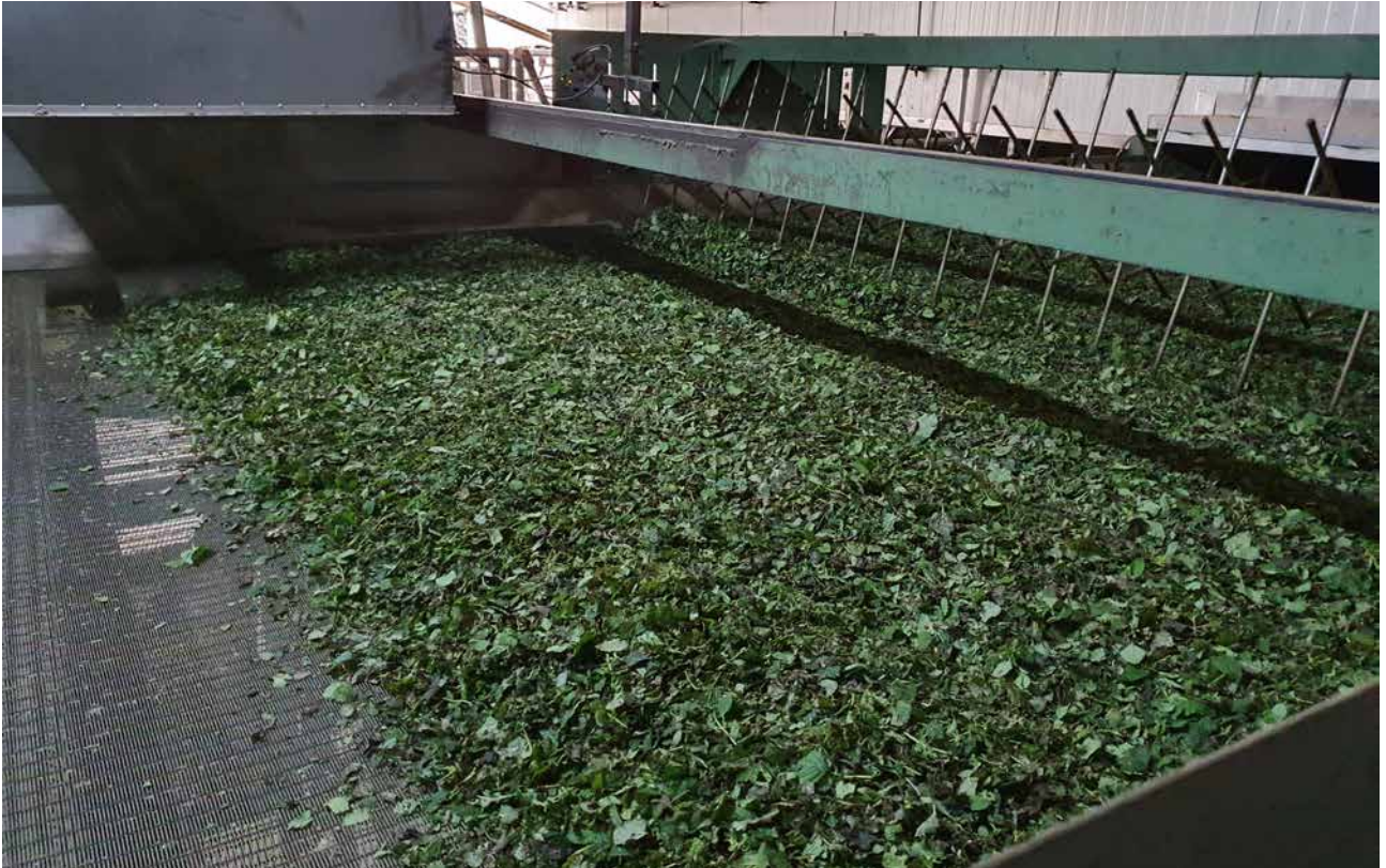
Herbs and spices drying on the bar mesh belt, Type: N 600
