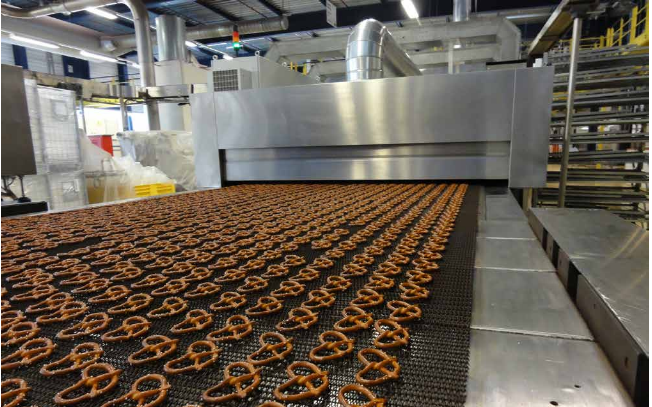
Pretzels on the balanced wire belt, Type: N 400
